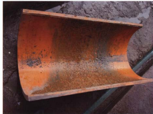
Lower haft of a damaged COMPAC bearing (not from Te Mana ) showing hydrolysis in centre of bearing due to lack of coolant. This bearing was used for another 10,000 miles after damage occurred.
