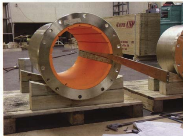
Brand new COMPAC bearing, showing the split-bearing system with a single key allowing remove and replacement of hafts with shaft in place. Note that water-ways are cut in top half only; water is carried around by the spinning shaft to form a hydrodynamic seat.
