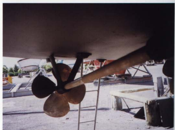
Trouble with water lube bearings, open to the sea, is that they are vulnerable to stray nylon and marine growth. Failure requires dry-docking.
