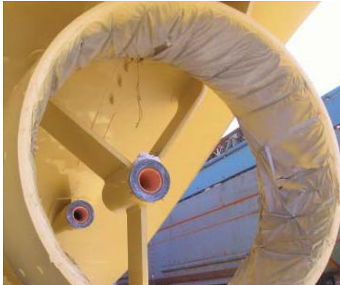
Seawater lubricated COMPAC propeller shaft bearings eliminate stern tube oil pollution
