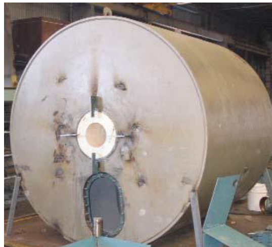
Seacor Marine stern roller installed with Thordon SXL bearing
